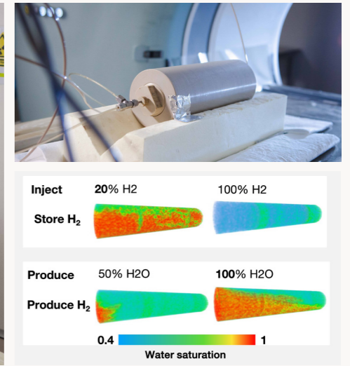
Core-flood experiments for Underground Hydrogen Storage, an example of many mCT & CT-based hydromechanics research conducted in our lab.
